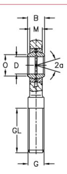
$\begin{array}{lll} A & = 102 \\ a \ (degrees) & = 7 \\ B & = 32 \\ D & = 45 \\ Dynamic \ drive \ (kN) = 127 \\ F & = 163 \\ g & = M42x3 \\ GL & = 94 \\ \end{array}$
